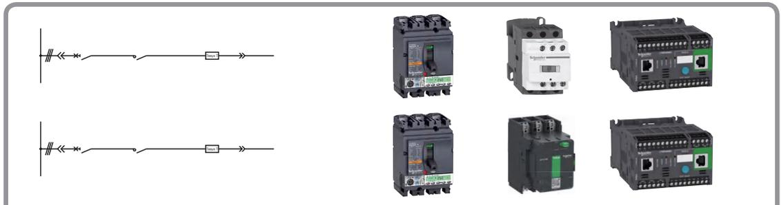
The image shows two schematic diagrams of a motor control circuit. The top diagram shows a three-phase supply connected to a three-phase motor through a circuit breaker and a contactor. The bottom diagram shows a similar setup but with a thermal relay (LTM) integrated into the contactor assembly. To the right of the diagrams are six photographs of the physical NSX 100-630 motor control units, showing various configurations and sizes.
